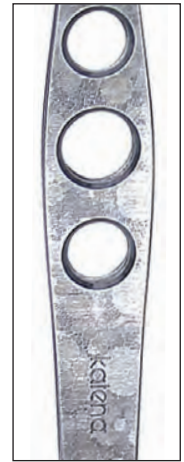
spots caused by mineral deposits
